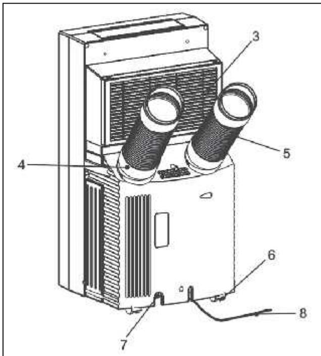
3. Evaporator air intake / air filter
