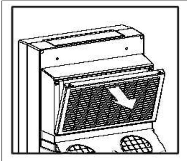
2. Remove the Pre-Filter from the filter frame.
