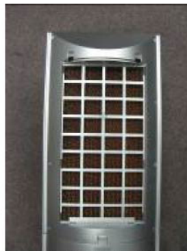
Honeycomb filter behind the back panel
