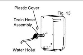
2. Insert the 16 ft. pump drain hose (included) into the bottom pump drain outlet (See Fig.14), then lead the drain hose to a suitable drainage facility. Make sure that the hose is fully inserted to avoid water leakage and no kinks which will cause the water to stop flowing.
