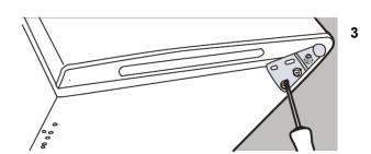
4. Screw the bottom hinge into place on the new side. Replace the leg on the other side.
