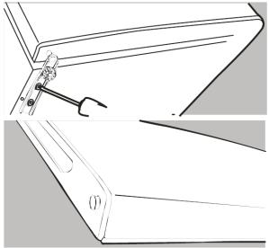
2. Remove the top hinge cover from door first. Then unscrew the two screws from top door hinge and replace on the other side.
